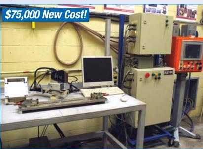
SERVO ROBOT SEAM FINDING & TRACKING SYSTEM, MODEL PILOT
