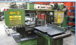
HYD MECH SEMI AUTO HORIZONTAL BANDSAW MODEL S20P
