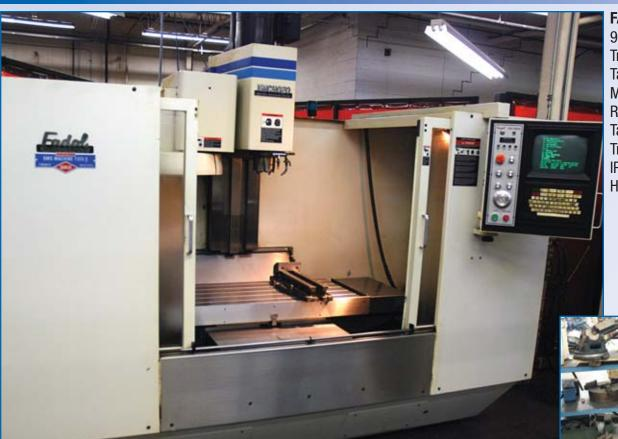
FADAL VMC 4020HT, Model 906-1, CNC 88HS Controls, Travels: X-40" Y-20" Z-20" Table Size 47.94" x 20", Max Spindle Speed 10,000 RPM, Cat 40, 21 ATC, Max Table Load 1,500 lb, Rapid Traverse X&Y 700, Z-600 IPM, Flood, Mist, RS232, 15 HP, 230/440V, sn 9606761
